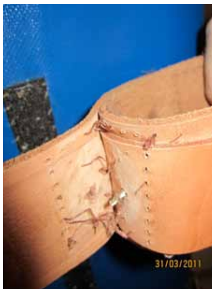
The restraint bed in a state of disrepair – note the nail protruding out of the wrist cuff, and the broken stitching.
