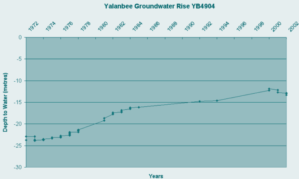
Figure 8. Long term groundwater trends in a bore at CSIRO's Yalanbee Research Station in Bakers Hill.
