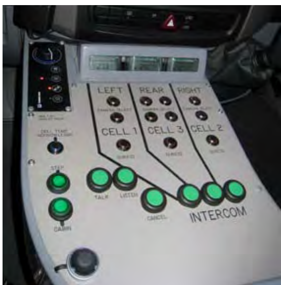
Audible temperature alarms, audible duress alarms, and intercom systems were retrofitted in existing vehicles. All already had video monitors. This is the cell monitoring and communications panel in a new vehicle.
