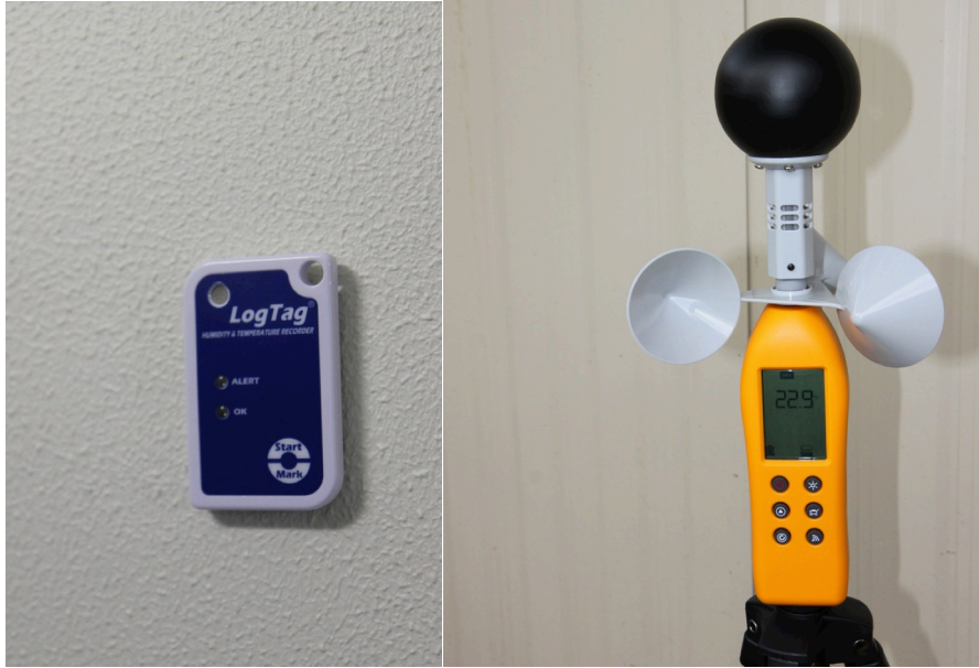
Figure 8 Logtag data logger and weather station used for temperature measurement
